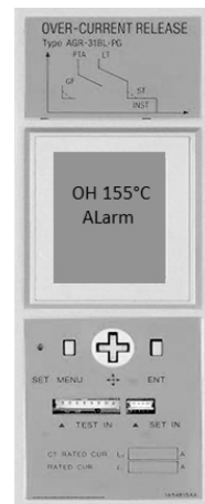
Figure 10 Protection Relay with Contact Temperature Monitor
